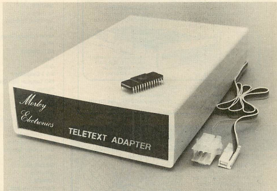
Figure 1. A popular teletext adaptor suitable for network use.
